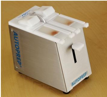
**STEP 4-** After the timed pause (approximately 2-3 seconds) to let the blood spread laterally and “wet” the glass blades side to side, the spreaders then pull the blood gently along the slide. Remove slides, prepare for staining and review.
