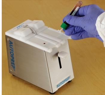
**STEP 2-** Place a blood drop on slides at target locations. Size of drop should be about pencil diameter (4 to 7mm).
