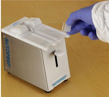
**STEP 1-** Place slides on platen; both right and left side. Make sure there is always a slide in place in both trays, even if not being used for a smear.
