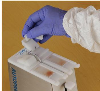
**STEP 5-** To clean spreaders rotate backward to rest position and wipe with tissue dampened with water. Make sure spreaders are dry before using.
