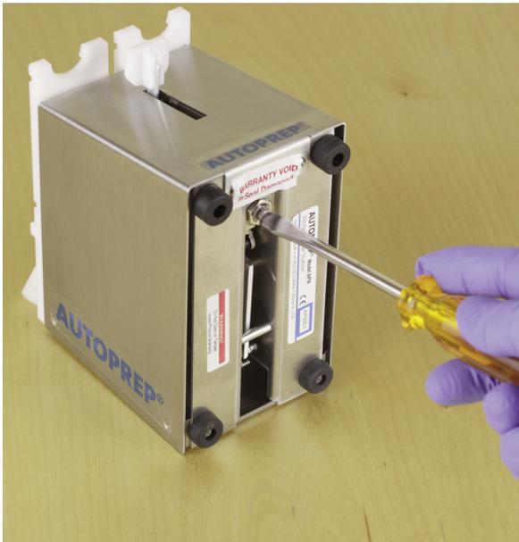
rotate the screw counterclockwise
